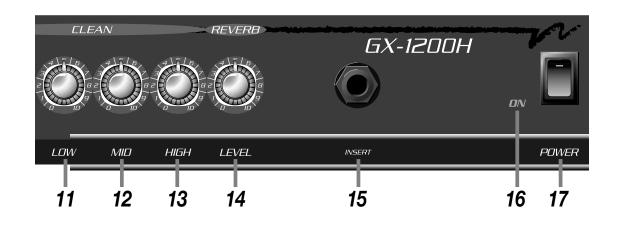
**15: INSERT:** Connect an external effects device via this jack. Use a stereo 1/4" male Y-cord: ring = send, tip = return, sleeve = ground. See the illustration on the panel to the right for more information
